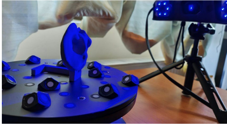
Fig. 2. 3D scanning of the prints with markers for point clouds alignment
